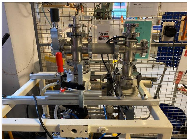
Fig. 3: Setup for testing the filtering function of the graphene membrane (under construction)
