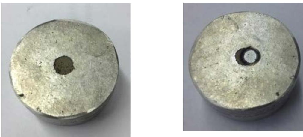
**Figure 2.** Mounted sample from an incinerator lab simulation, before (left) and after (right) sputtering in the GD. Note that in this figure the sputter spot is 4 mm, in the major part of the project a 2 mm spot was used.
