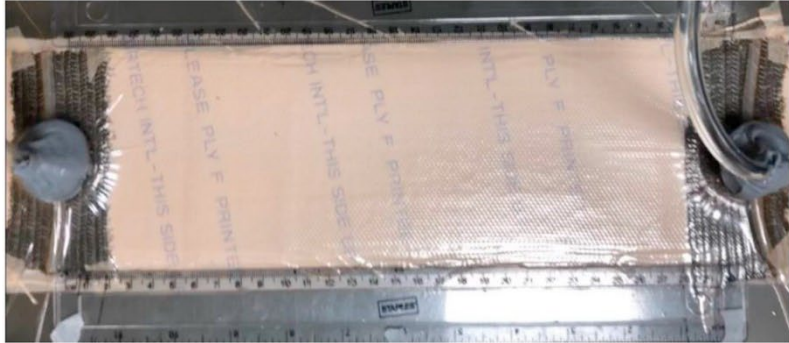
Figure 4. Resin infusion setup and the mean data for the infused composite plate.
