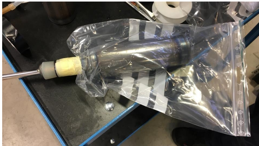
Figure 14 - Helium leak test of a HIP-capsule.
