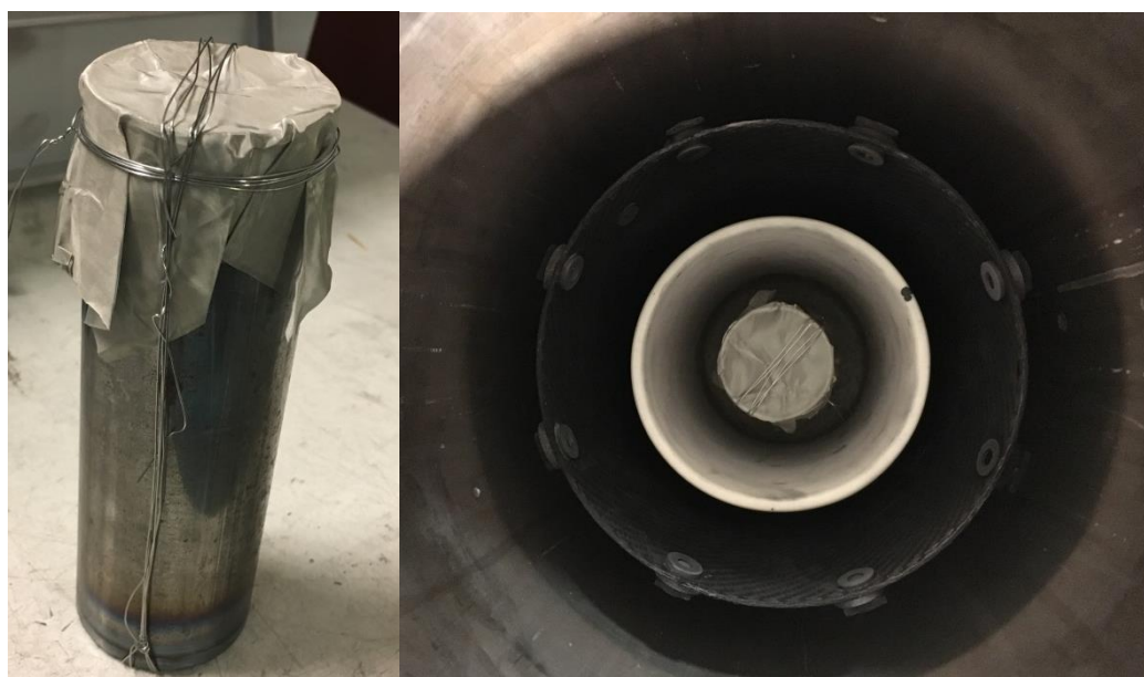
Figure 10 – Mesh covered container used in the fill experiments (left). Container placed in the HIP furnace (right).
