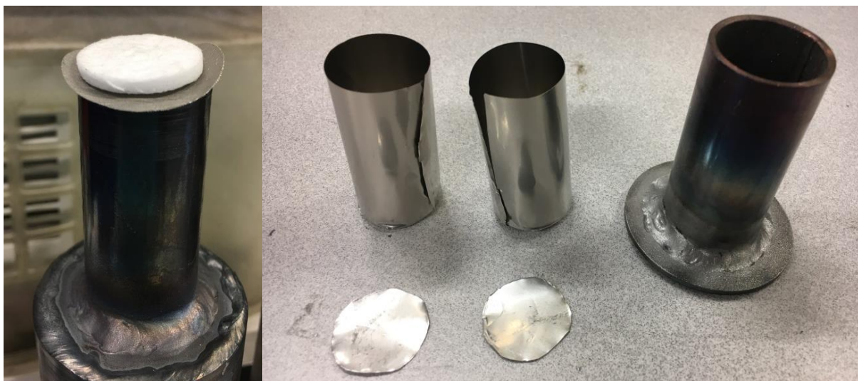
Figure 15 – Bottom pair of ceramic wool disc and mesh before pushing them down into place (left). On top of the pair, stainless steel foil cups with an extra bottom sheet were inserted into the fill pipe (right). The cups were then filled with the hydrogen filled microspheres. An inverted pair was then placed above the filled foil cups.
