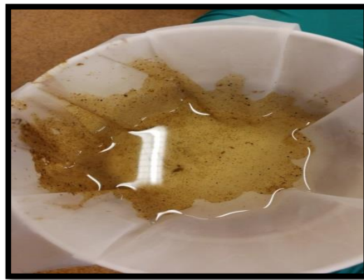
Figure 22- Screen clogging on the Wastewater effluent
