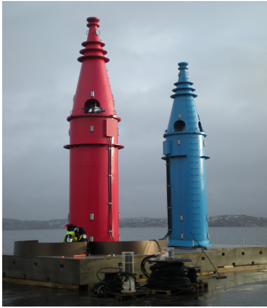
Oscillating bodies (submerged), Taut-moored system, Uppsala University's concept, Sweden
